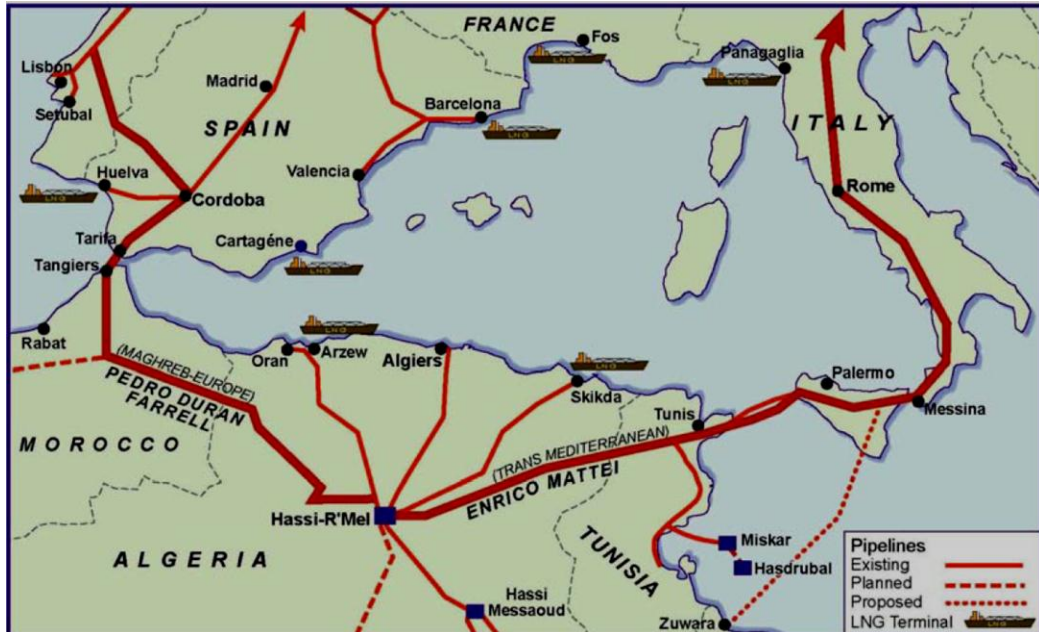
Figure 5.1 Transmed and Maghreb-Europe Gas Pipelines
